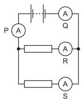
Which of these ammeters show the greatest reading?
